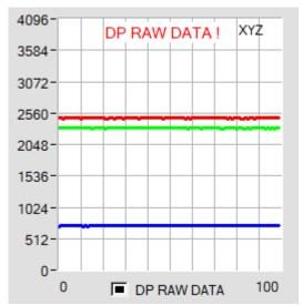
To understand with which **X**, **Y** and **Z** values the sensor works in parameter set 2, you can display this raw data in the display **XYZ** using the **DP RAW DATA** check box.
